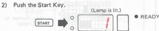
This indicates the needle selection for the first row needs to be done.
